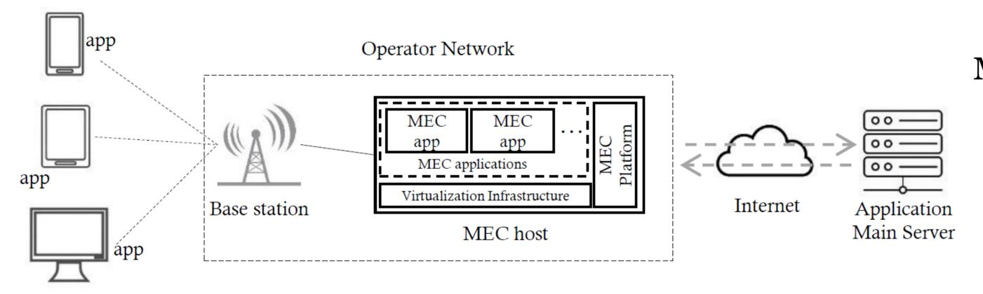
MEC is one of the emerging key technologies in 5G Mobile Networks, providing reduced end-to-end latency for applications and reduced load in the transport network.
