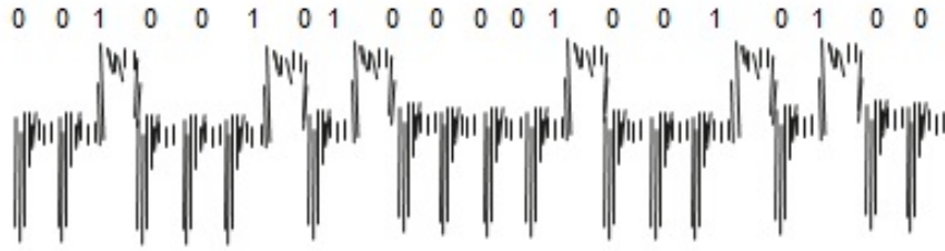
Figure 20: Illustration of a power trace of a modular exponentiation operation, adapted from (Paul Kocher, Jaffe, Jun, and Rohatgi, 2011).
